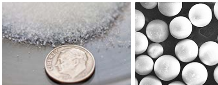
Looking like microscopic pearls, NETL's BIAS technology enables the capture of CO 2 in large-scale processes.
